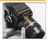
C. The accessory, with lens attached to it, is attached to the body in the same manner that the lens is attached. First, rotate the film winding crank and cock the lens shutter. Next, align the orange dot on the body with the red dot on the accessory and insert the latter. Finally, rotate counter-clockwise fully, until there is an audible click which will indicate attachment.
