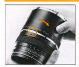
B. To attach the accessory to the lens, align the orange dot on the accessory with the red dot on the lens and insert the latter. Then, rotate in the counter-clockwise direction until there is an audible click, which will indicate attachment.
