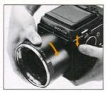
C. In order to detach the accessory from the body, press the lens release button (on the left side of the body) down and, at the same time, rotate the accessory in the clockwise direction until it makes a full stop and can be detached.
